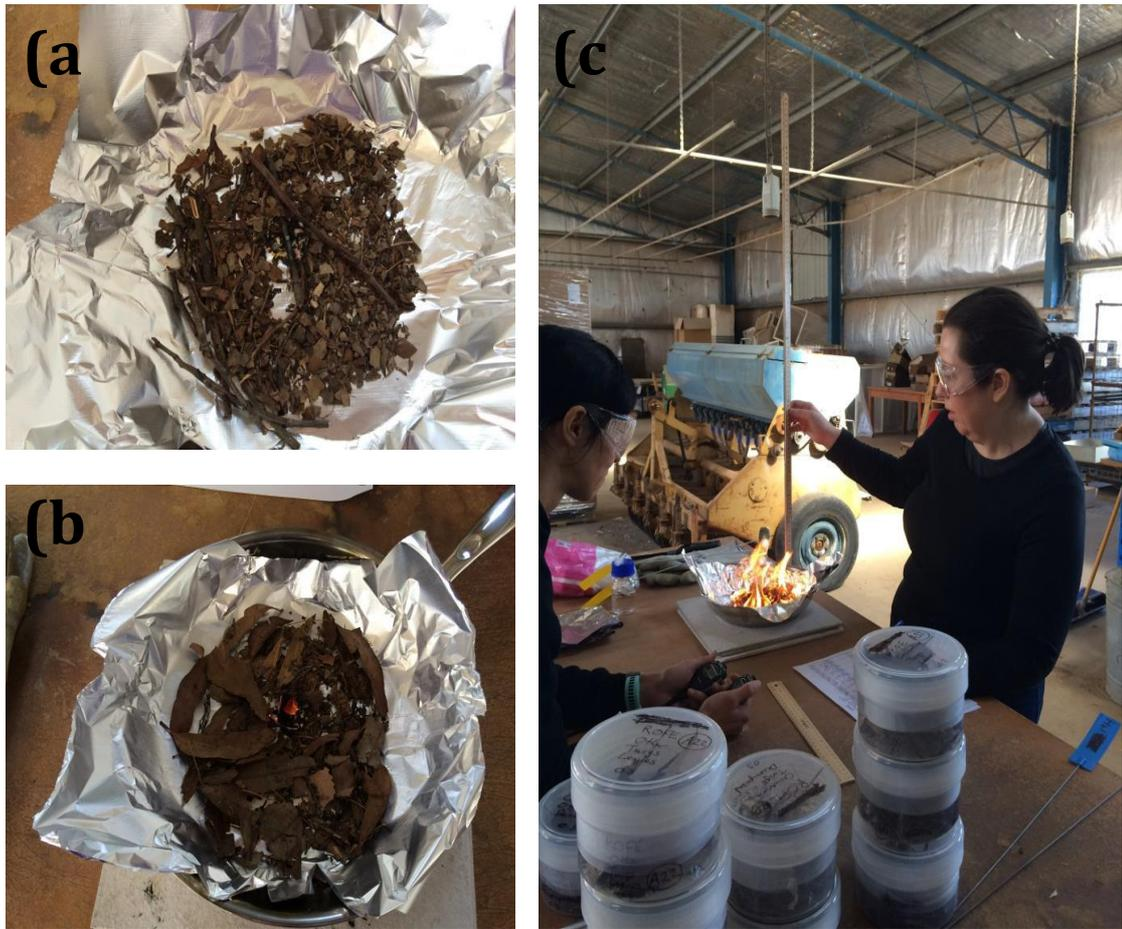
**Figure 3.2** Examples of litter mixtures prior to burning: (a) twigs and decomposed material, and (b) leaves and decomposed material, and (c) measuring flame height.
