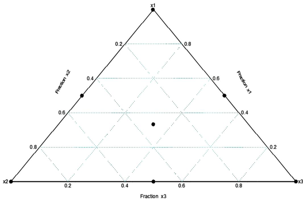
**Figure 3.1** Simplex Centroid Design with three components (Source: Lawson and Willden 2016).
