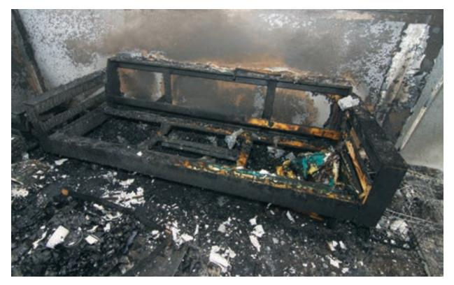
The room with no sprinkler and its synthetic, flammable contents were completely destroyed during the demonstration burn.
