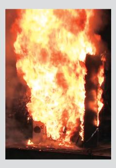
FIGURE 2. NMC fire development during largescale free burn test: near time of ignition (left), near time of predicted spreation (centre), peak heat release rate (right).
