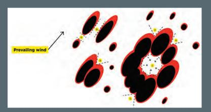
FIGURE 1. Schematic representation of coalescing spot fires and the different forms of fire line interaction between individual spots. Examples of fire line interactions include (a) intersecting oblique lines, (b) non-intersecting converging fire edges, and (c) collapsing or constricting
