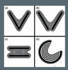
FIGURE 2. Examples of output from the pyrogenic potential model for different initial fire line geometries: (a) junction fire (v-shaped fire); (b) separated v-shaped fire; (c) two parallel fire lines; (d) a closed (270°C) arc. The black and white banding indicates the spread of the fires over equally spaced points in time, so thicker bands correspond to relatively higher rates of spread.
