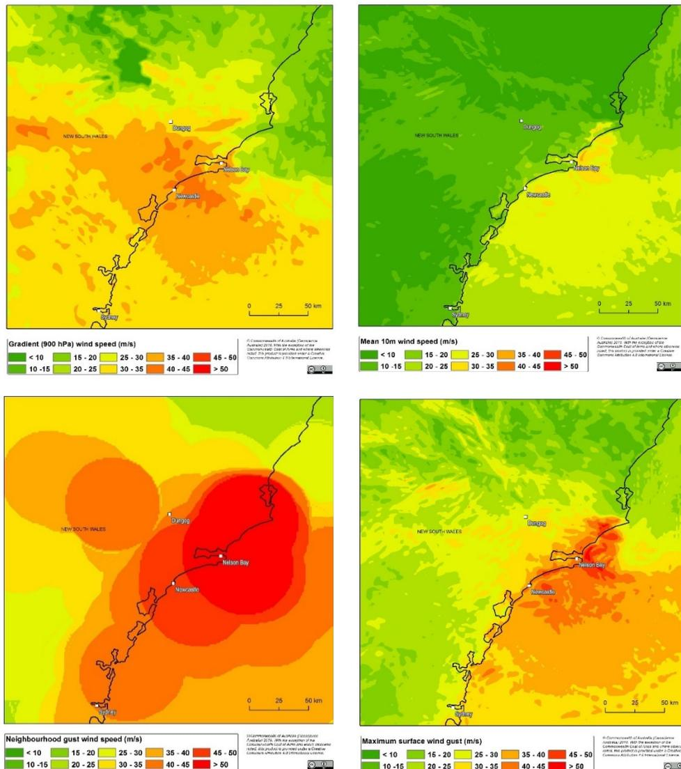
Figure 2: Four characterisations of wind hazard for the 2015 East Coast Low event, as simulated in the BARRA-SY reanalysis (clockwise from top left): point gradient wind speed, point mean wind speed, point gust wind speed and neighbourhood gust wind speed. All values are in units of metres per second.
