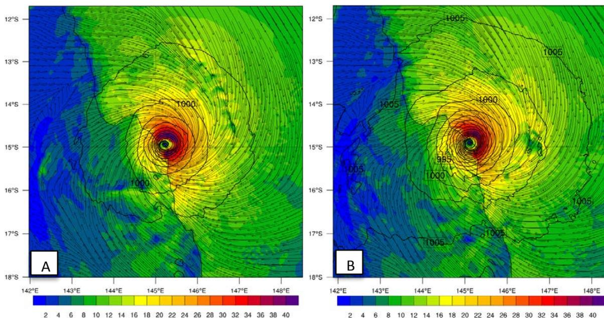
FIGURE 2. WIND SPEED AND PRESSURE FIELDS FOR THE 3.3 KM WRF-ARW RESOLUTION TC ITA AT LANDFALL. COLOURED CONTOURS INDICATE THE 10 M WIND SPEED MAGNITUDE, ISOBARS ARE DISPLAYED WITH SOLID BLACK LINES, AND WIND DIRECTION WITH ARROWS.
