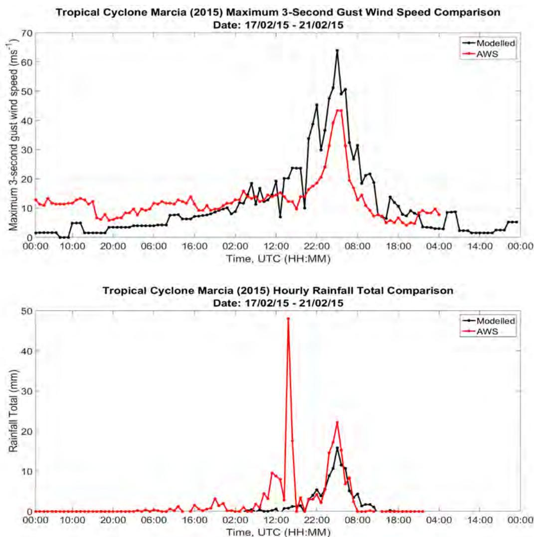
FIG. 2. COMPARISON OF SIMULATED (BLACK) VERSUS OBSERVED (RED) HOURLY MAXIMUM THREE-SECOND GUST WIND SPEEDS (TOP) AND RAINFALL TOTALS (BOTTOM) AT THE YEPPOON THE ESPLANADE AWS.
