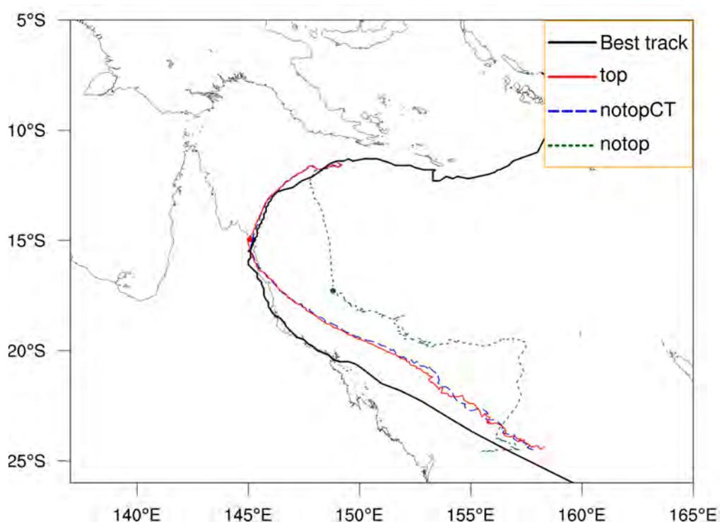
FIGURE 1. WRF MODELLED TRACKS AND BEST TRACK (BLACK) OF TC ITA. WRF DEFAULT PHYSICS MODELLED TRACK (RED), TOPOGRAPHY SET TO ZERO FOR THE ENTIRE DOMAIN (GREEN), AND TOPOGRAPHY TURNED OFF FOR THE COOKTOWN AREA ONLY (BLUE). LANDFALL POINTS ACCORDING TO THE BEST TRACK LANDFALL TIME ARE INDICATED WITH COLOURED DOTS.
