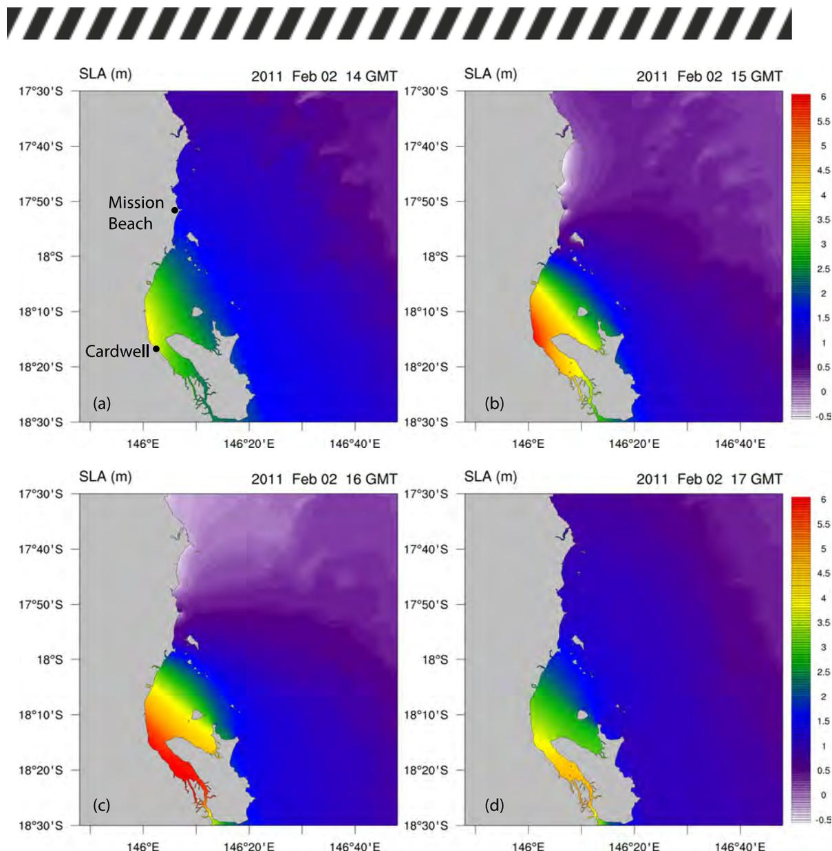
FIGURE 2. SIMULATED STORM SURGE AT CARDWELL SHOWING THE PROPAGATION OF THE SURGE INTO THE BAY FOLLOWING THE CYCLONE CROSSING THE COAST NEAR MISSION BEACH JUST AFTER 14:00 (GMT). HEIGHT COLOUR SHOWN IN METRES.
