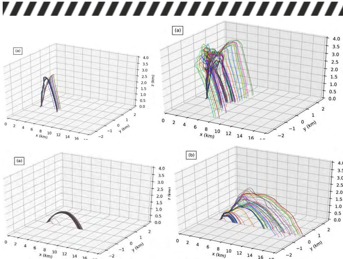
FIGURE 2. TRAJECTORIES OF 100 FIREBRANDS LOFTED BY THE MEAN (LEFT) AND TIME-VARYING (RIGHT) PLUMES UNDER BACKGROUND WIND SPEEDS OF 5 (TOP) AND 15 (BOTTOM) M S<sup>-1</sup>.
