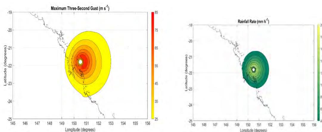
FIGURE 1. TC MARCIA SIMULATED HOURLY MAXIMUM THREE-SECOND GUST WIND FIELD (LEFT) AND RAINFALL RATE (RIGHT) FIELDS GENERATED AT APPROXIMATELY TWO HOURS BEFORE LANDFALL (19 FEBRUARY 2015 AT 20:00 UTC).
