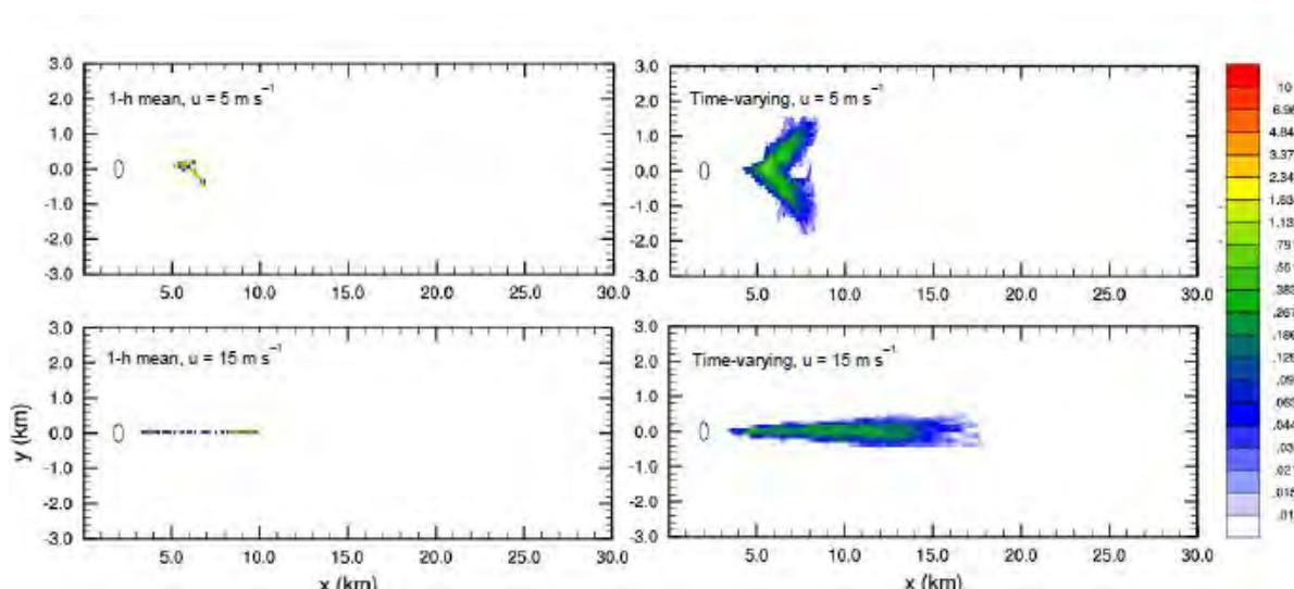
FIGURE 3. SPATIAL DISTRIBUTIONS OF FIREBRAND LANDING POSITION (PERCENT OF PARTICLES LAUNCHED PER KM<sup>2</sup>) FOR THE MEAN (LEFT) AND TIME-VARYING (RIGHT) PLUMES UNDER BACKGROUND WIND SPEEDS OF 5 (TOP) AND 15 (BOTTOM) M S<sup>-1</sup>.
