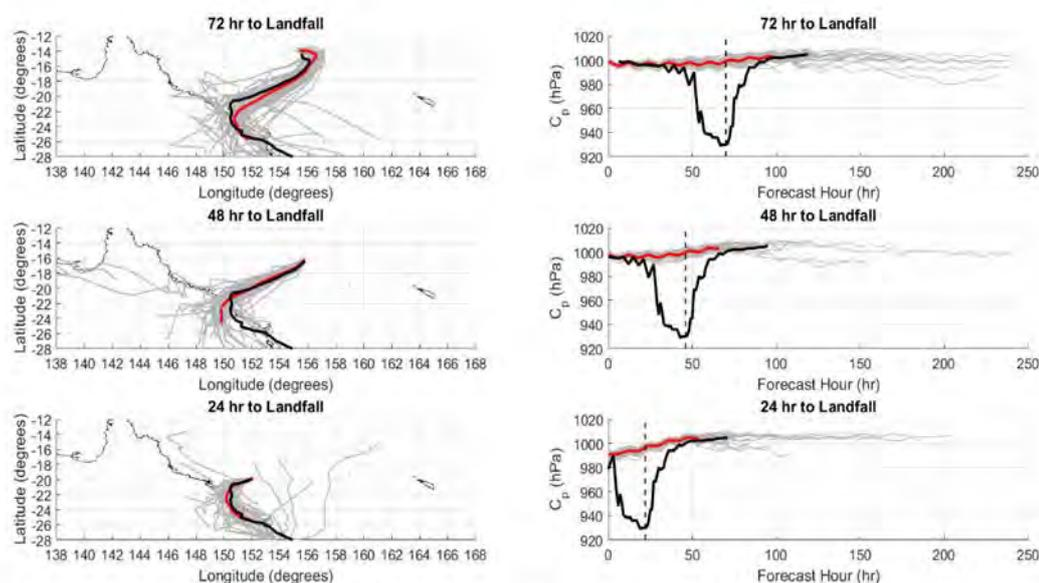
FIG. 3. ECMWF EPS FORECAST MEMBER (GRAY LINES) AND ENSEMBLE MEAN (RED LINE) TRACK AND MINIMUM CENTRAL PRESSURE FORECASTS 72-, 48-, AND 24-HR LEADING UP TO THE LANDFALL OF TC MARCIA. THE BLACK LINE REPRESENTS THE BOM BEST TRACK POSITION AND MINIMUM CENTRAL PRESSURE.
