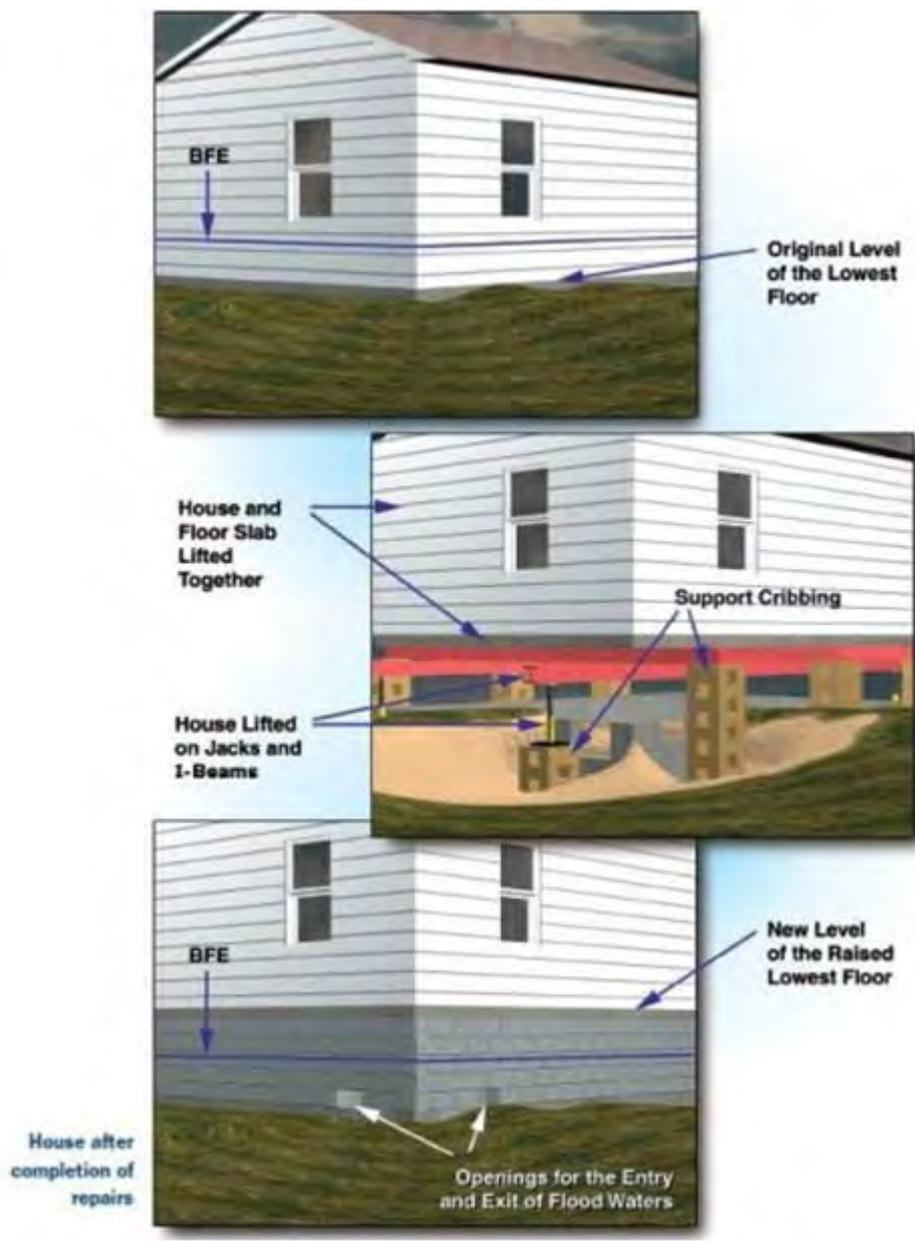
FIGURE 2: TECHNIQUES FOR ELEVATION (FEMA, 2000)
