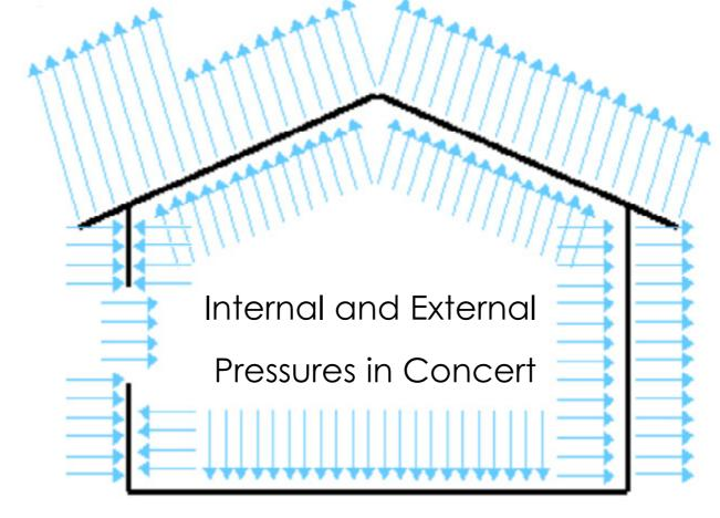
Results showed that the Australian standard slightly loading wind underestimates the positive internal pressure in the nominally sealed buildings, but over-estimates the internal suction pressure by 90%, usually the critical design case for nominally sealed buildings.
