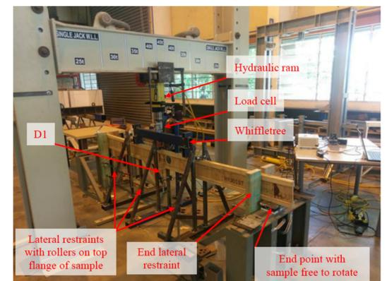
Figure 3: Four Point Bend Test Setup
