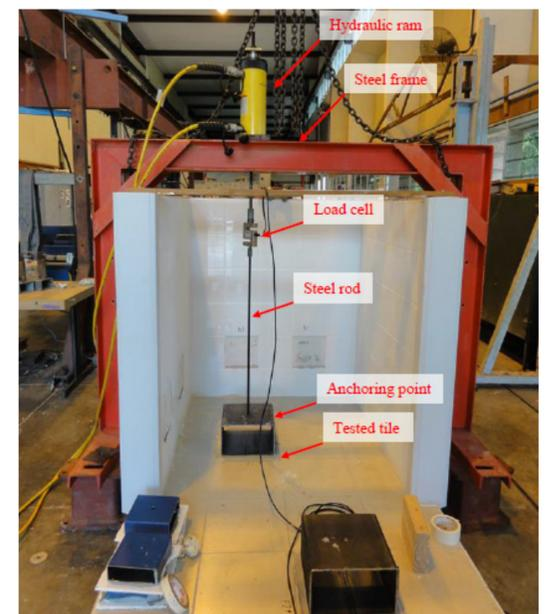
Figure 2: Floor Tile Hydraulic Test Setup
