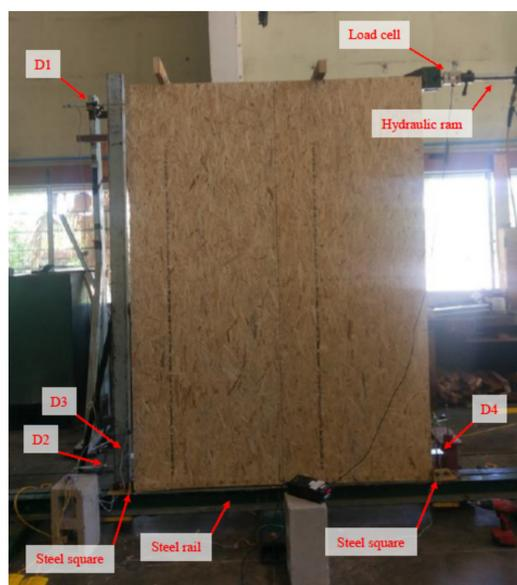
Figure 1: Racking Strength Testing Frame
