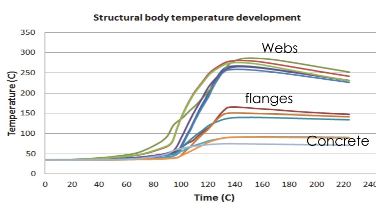
**Model 3:** Crown+surface fuel model, Wind velocity at 10m from ground is 2m/s
