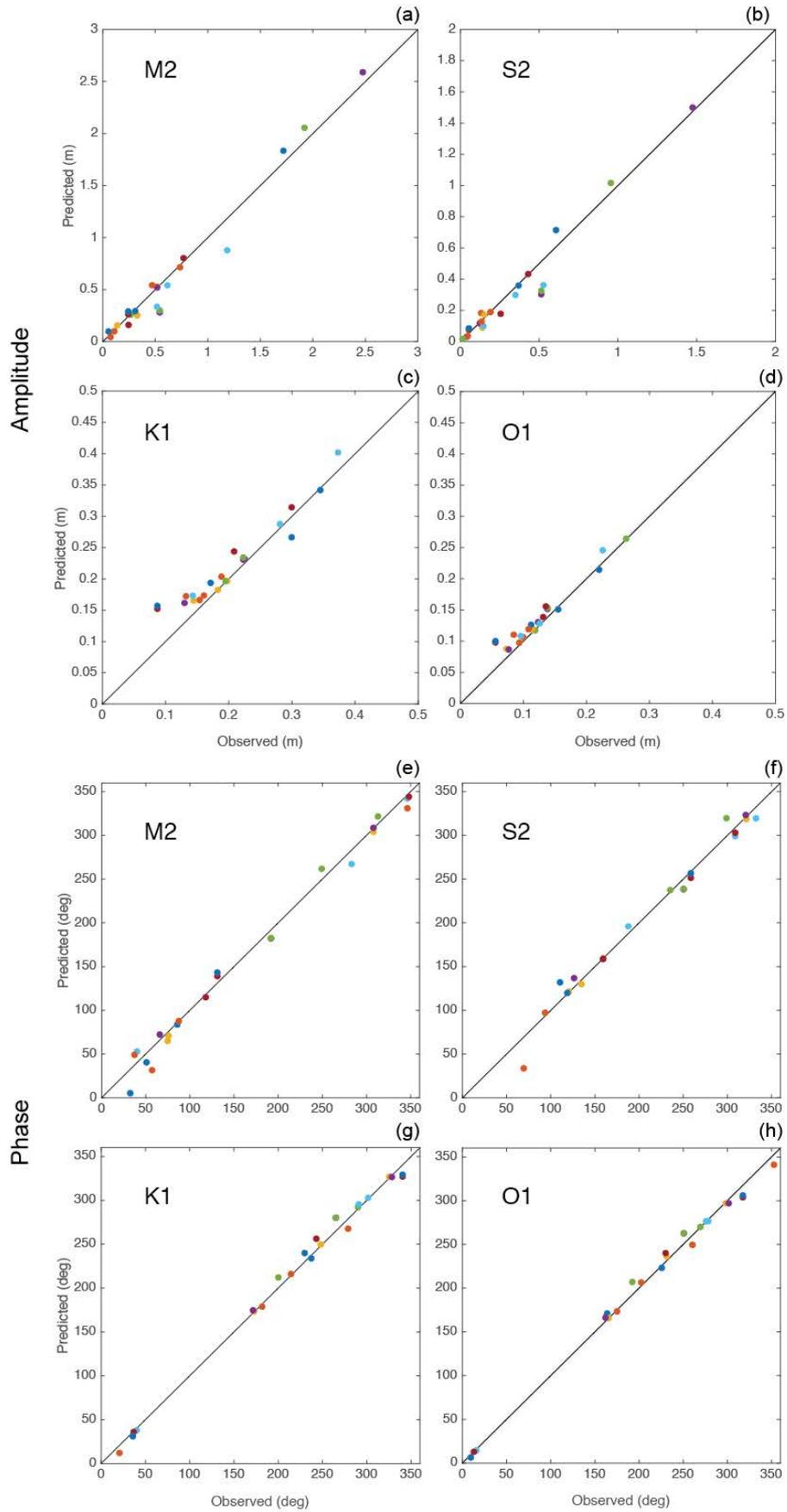
FIGURE 4. OBSERVED VS. PREDICTED AMPLITUDE (A-D) AND PHASE (E-F) OF THE FOUR MAIN TIDAL CONSTITUENTS AT 28 TIDE GAUGE SITES OBTAINED THROUGH HARMONIC ANALYSIS OF PREDICTED AND OBSERVED TOTAL WATER LEVELS.
