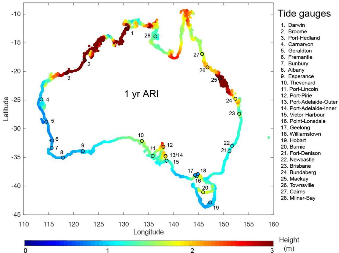
FIGURE 3. LOCATION OF TIDE GAUGE SITES USED FOR VALIDATION OF SCHISM STORM SURGE MODEL OVERLAPPED ON PREDICTED 1 YEAR AVERAGE RECURRENCE INTERVAL AS AN INDICATOR FOR TIDAL RANGE AROUND AUSTRALIA.
