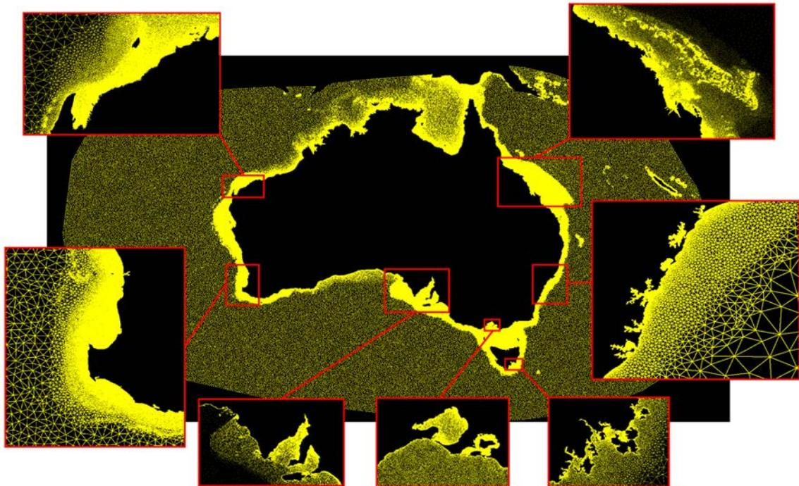
FIGURE 1. SCHISM NUMERICAL MODEL DOMAIN WITH SUBSETS ILLUSTRATING HIGHER RESOLUTION AT THE COAST. SPATIAL RESOLUTION AT THE COAST RANGED FROM 100 TO 800 METRES AND DECREASED OFFSHORE.
