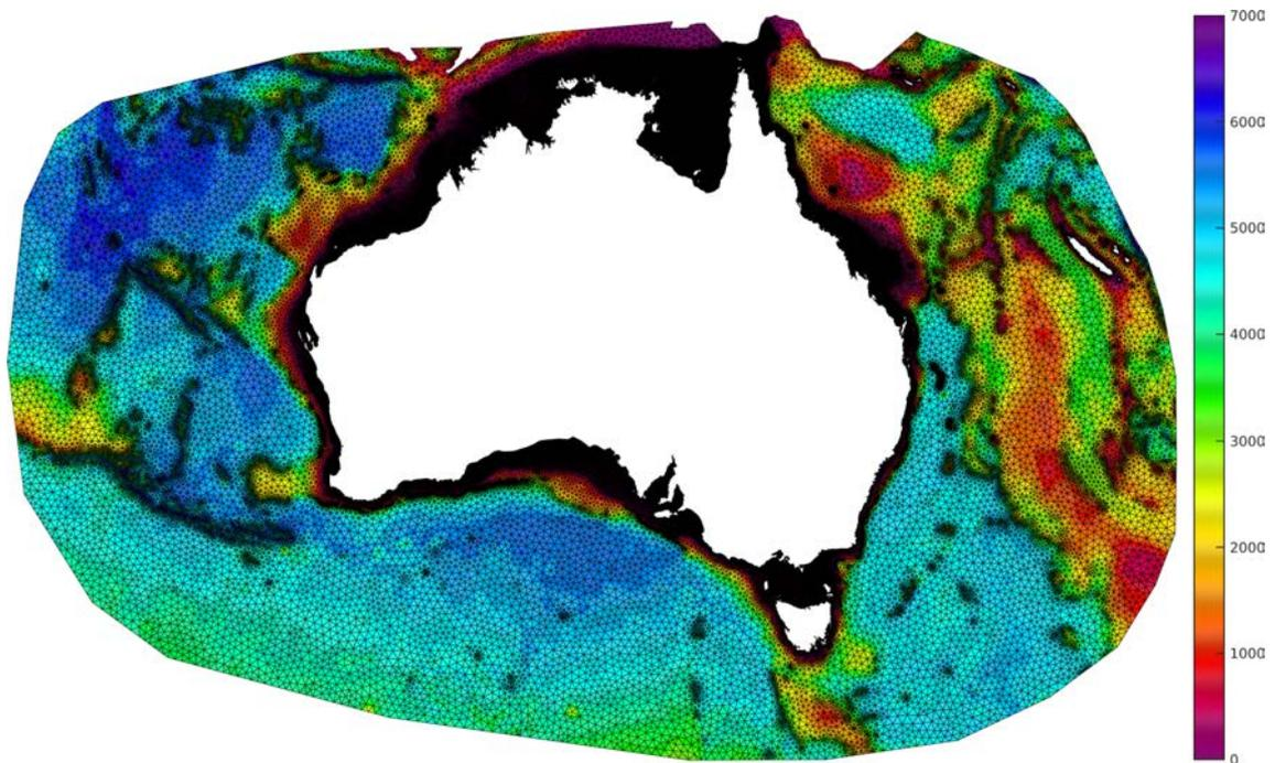
FIGURE 2. SCHISM UNSTRUCTURED MODEL MESH WITH COLOURS INDICATING DEPTH IN METRES.
