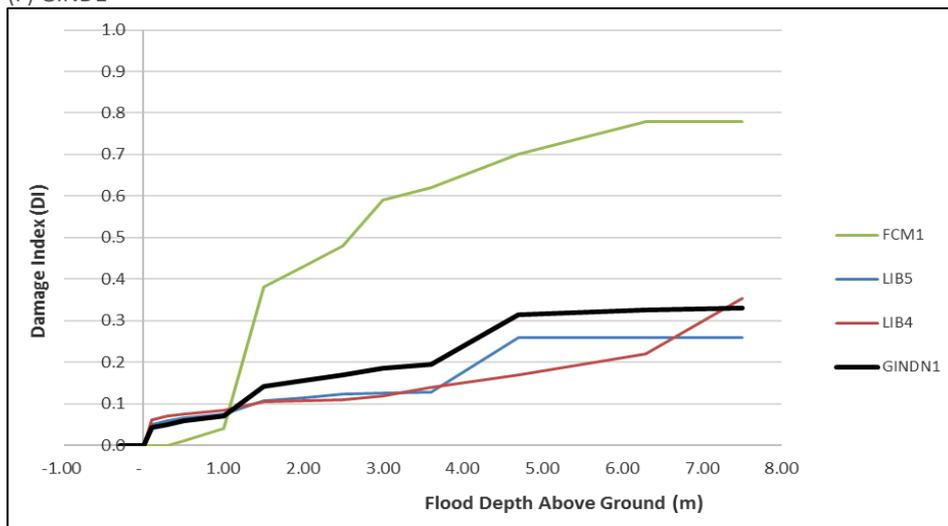
Figure 5: Flood Vulnerability functions: detailed and generalised (cont.).
