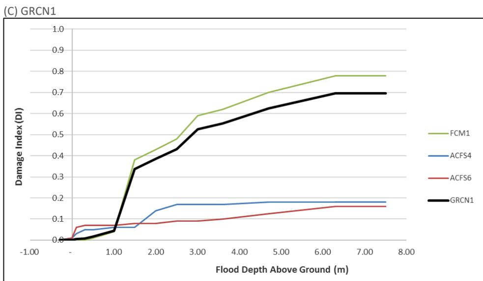
Figure 5: Flood Vulnerability functions: detailed and generalised.
