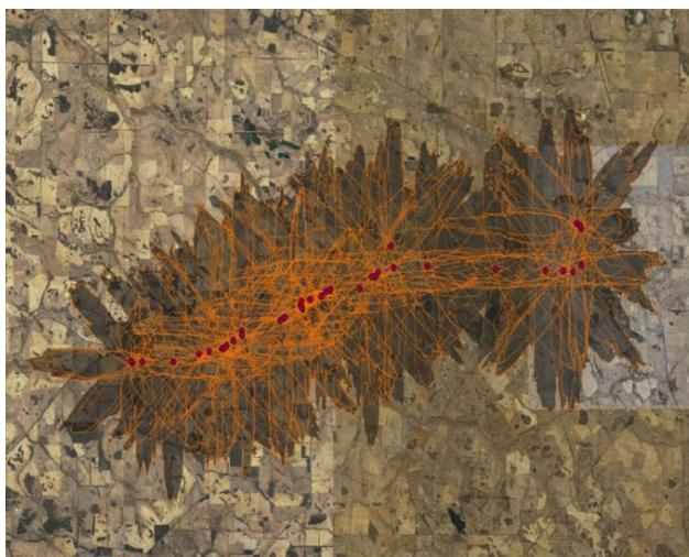
Figures 4 & 5: Example of fire runs modelled on 1 cardinal wind directions and further processing in the AWS to produce 8 cardinal wind directions from Western Power above ground power poles.
