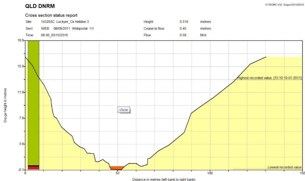
Figure 3.11: River profile of Lockyer Creek at Helidon Number 3
