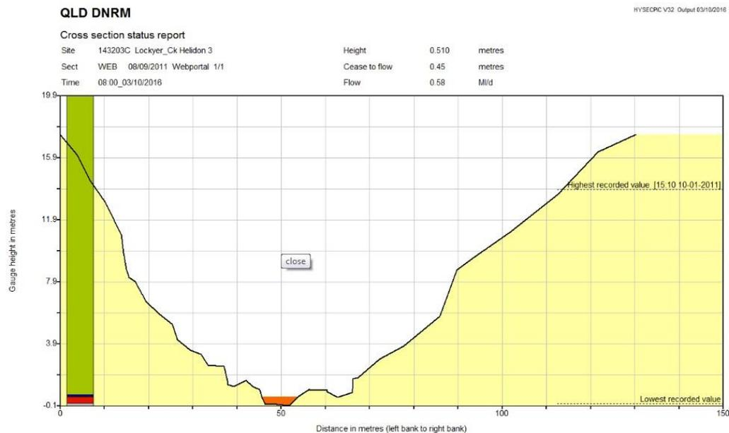
Figure 6.6: River profile of Lockyer Creek at Helidon Number 3
