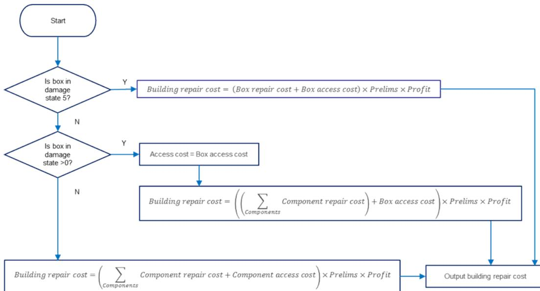
FIGURE 3 LOGIC USED TO ESTIMATE BUILDING REPAIR COST
