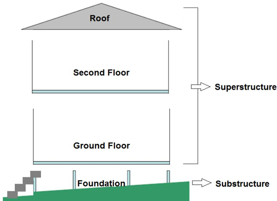
FIGURE 2: BUILDING STRUCTURE DIVIDED INTO MAIN COMPONENTS
