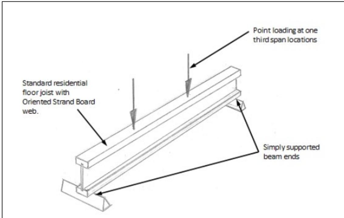
FIGURE 10: SCHEMATIC DIAGRAM OF ENGINEERED TIMBER JOIST IN FOUR POINT BENDING
