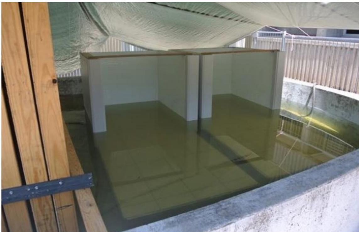
FIGURE 7: BATHROOM SAMPLES IN WATER TANK DURING FLOOD SIMULATION
