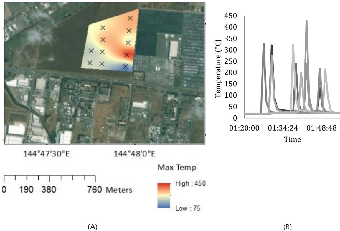
FIGURE 2 MAXIMUM TEMPERATURE RECORDED IN THE BURNED GRASSLAND AREA (A) AND TEMPERATURE REACHED BY EACH SENSOR OVER TIME (B).
