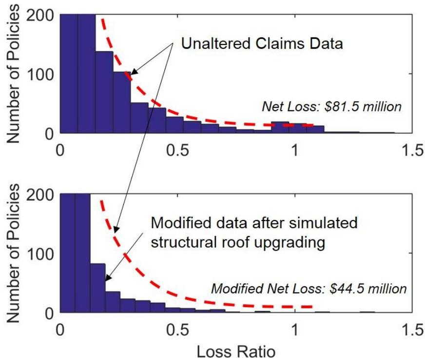
Figure 6. Claims data with and without the simulated effects of structural roof upgrades from Tropical Cyclone Yasi (2011) for residential housing constructed in the Queensland coastal region from 1960 to 1980
