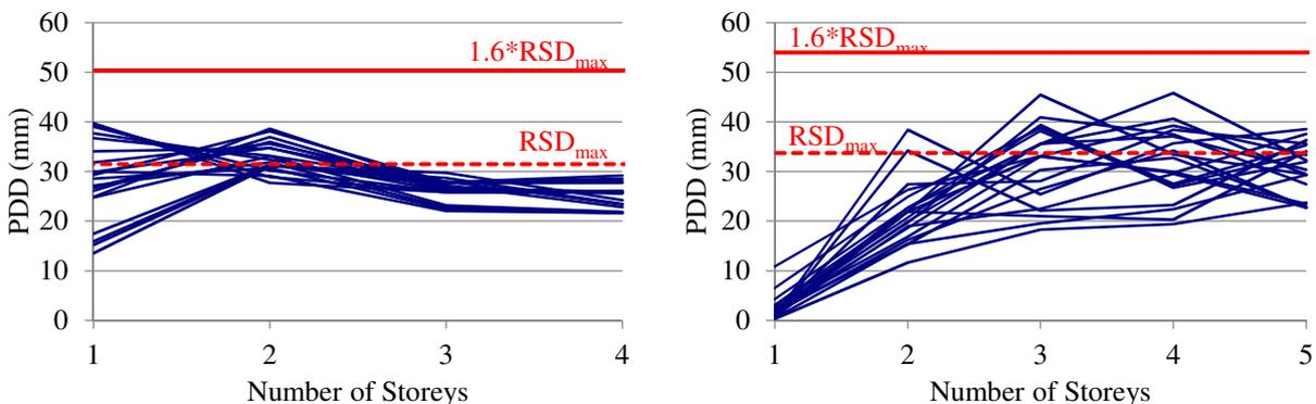
**Figure 4. PDD as a function of the number of storeys for different floor areas and for (a) building Type 1 and (b) building Type 2**
