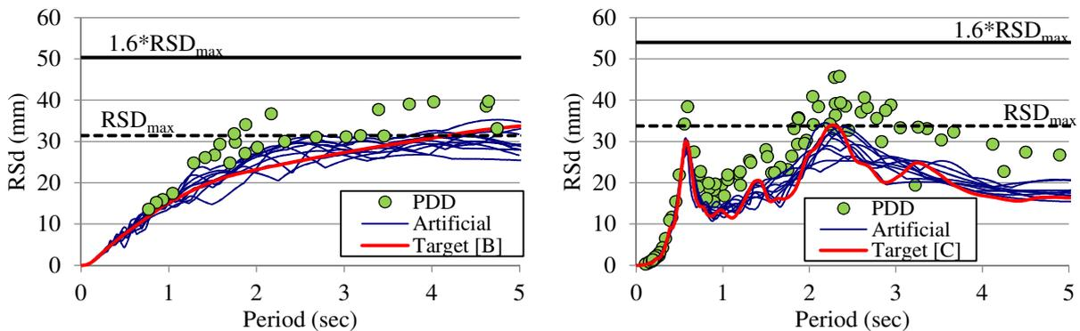
**Figure 3. Displacement response of artificial motions for (a) soil class B, building Type 1 and (b) soil class C, building Type 2**
