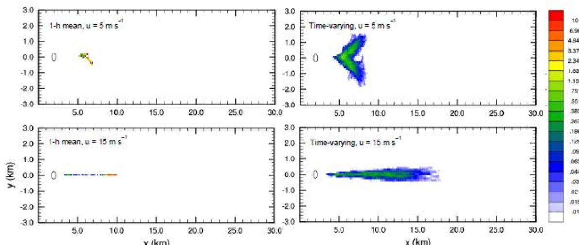
FIGURE 3. SPATIAL DISTRIBUTIONS OF FIREBRAND LANDING POSITION (PERCENT OF PARTICLES LAUNCHED PER KM<sup>2</sup>) FOR THE MEAN (LEFT) AND TIME-VARYING (RIGHT) PLUMES UNDER BACKGROUND WIND SPEEDS OF 5 (TOP) AND 15 (BOTTOM) M S<sup>-1</sup>.
