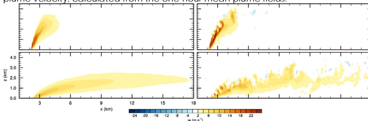
FIGURE 1. VERTICAL CROSS-SECTIONS OF THE MEAN (LEFT) AND INSTANTANEOUS (RIGHT) VERTICAL VELOCITY, M S<sup>-1</sup>, THROUGH THE PLUME CENTRE LINE, FOR BACKGROUND WIND SPEEDS OF 5 (TOP) AND 15 (BOTTOM) M S<sup>-1</sup>.
