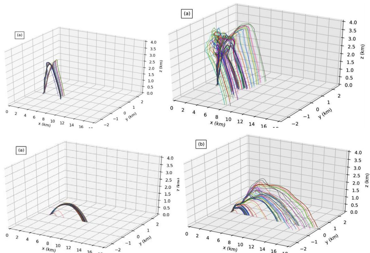
FIGURE 2. TRAJECTORIES OF 100 FIREBRANDS LOFTED BY THE MEAN (LEFT) AND TIME-VARYING (RIGHT) PLUMES UNDER BACKGROUND WIND SPEEDS OF 5 (TOP) AND 15 (BOTTOM) M S<sup>-1</sup>.
