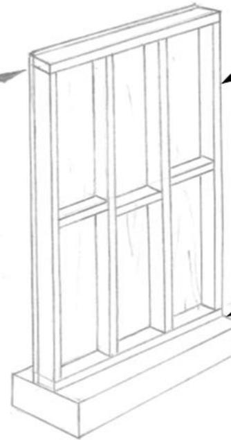
Timber framed wall to 2400mm height. Oriented Strandboard and/or HDF lining one face as per standard residential bracing panel.
