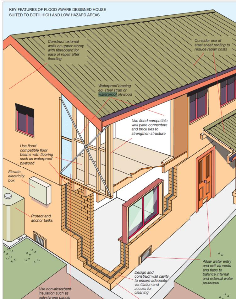
Figure 8 (Cont.). Techniques for wet floodproofing (FEMA, 2000)
