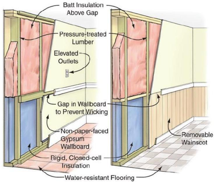
(C) Anchoring tanks, elevating utilities, using flood-resistant materials (HNFMSC, 2006)
