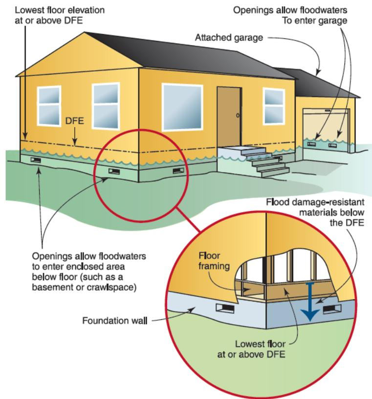
Figure 8. Techniques for wet floodproofing (FEMA, 2000)
