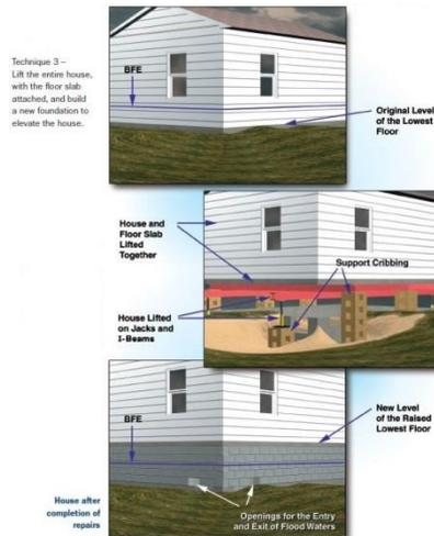
Figure 5. Techniques for elevating floor levels (FEMA, 2000)
