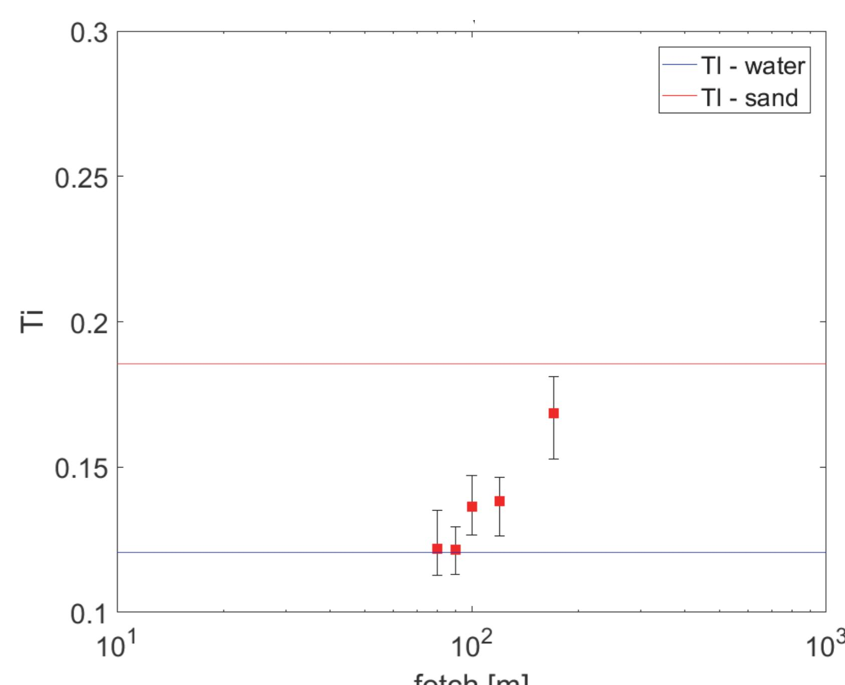
Figure 3: Turbulence intensity for wind speeds greater than 10 m/s measured at Hurricane Sandy (2012) StickNet tower 103A
